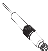
Measuring point Extensions 60 mm (not for 52 179-000/-601). Can be installed without draining of the system. AMETAL®/Stainless steel/EPDM
