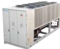
EWAD-C Family 620-2,000 kW R-134a Single - Screw with VFD
