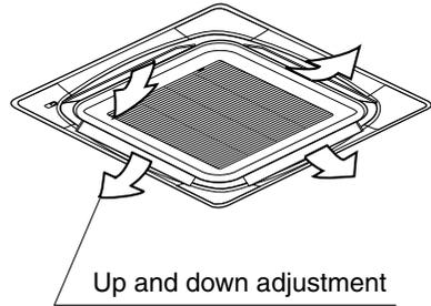
Press the **AIR FLOW DIRECTION ADJUST** button to select the air direction as shown below.
