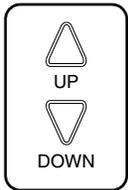
Each time this button is pressed, setting temperature rises 1°C.
