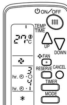
When the timer is programmed to stop the system after 3 hours and start the system after 4 hours, the system will stop after 3 hours and then 1 hour later the system will start.
