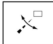
DISPLAY appears and the air flow direction continuously varies. (Automatic swing setting)
