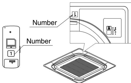
Operate the indoor unit with the remote controller of the same number.
