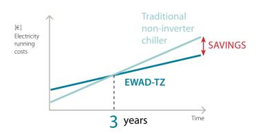
Based on: 1,500 working hours/year industrial electricity price = 0.17€/kWh design conditions 12/7°C evaporator and 35°C ambient
