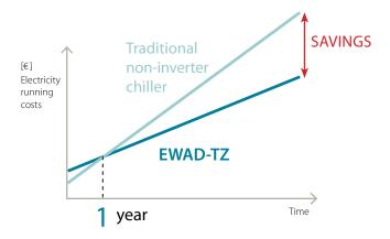
Based on: 5,000 working hours/year industrial electricity price = 0.17€/kWh design conditions 12/7°C evaporator and 35°C ambient
