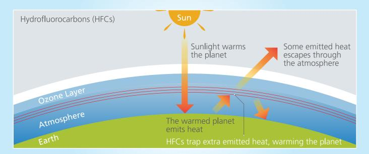
Hydrofluorocarbons (HFCs) are commonly used as refrigerants in residential air conditioner equipment. HFCs emissions increase the warming of the stratosphere, which speeds up the chemical reactions that destroy ozone molecules. Their impact on global warming can be many times greater than carbon dioxide (CO2).
