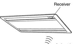
2 short beeps from the receiver indicates that the transmission is properly done.
