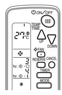
When the timer is programmed to stop the system after 3 hours and start the system after 4 hours, the system will stop after 3 hours and then 1 hour later the system will start.
